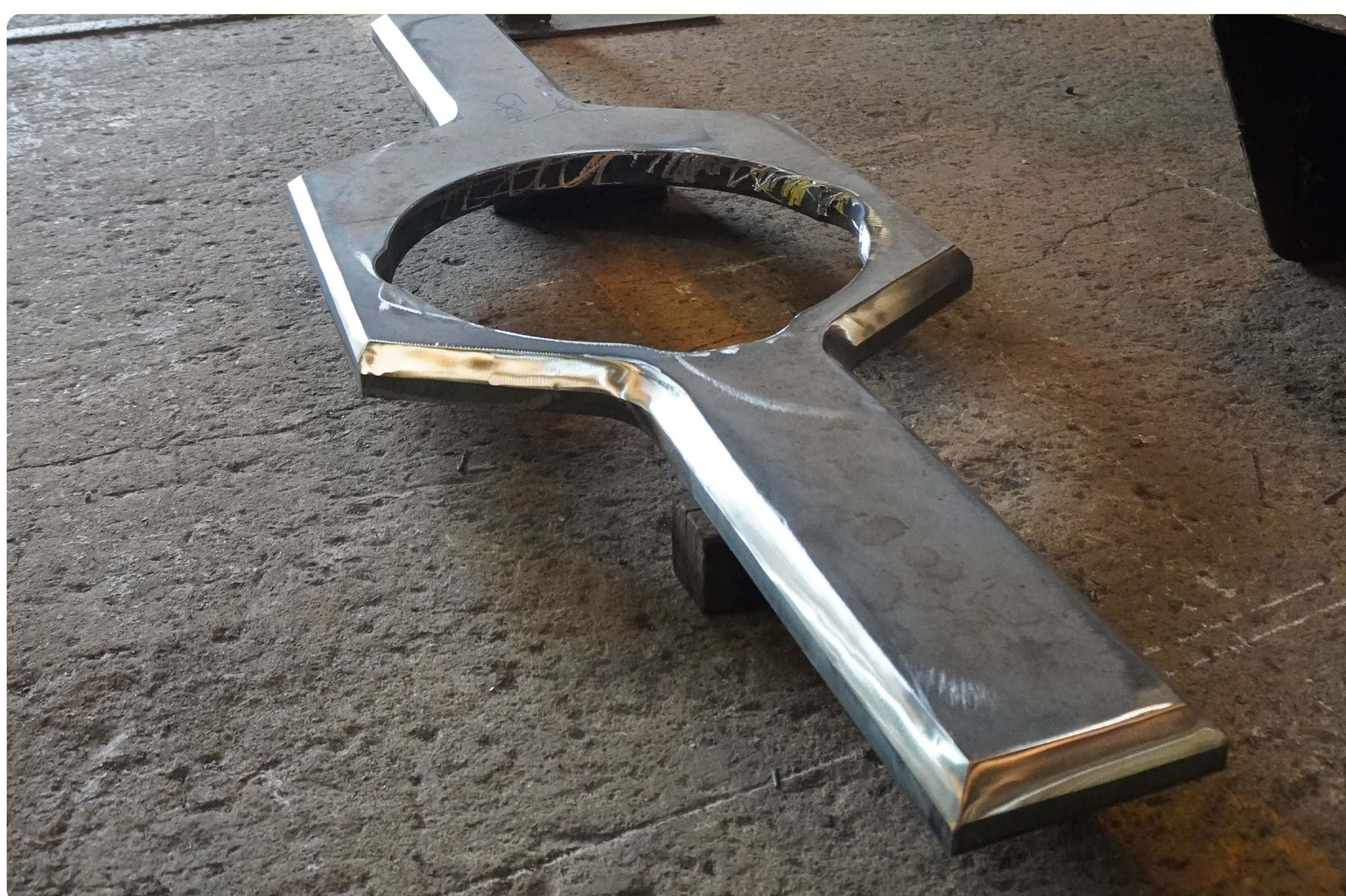
Cut and chamfered in Richards Bay
